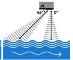
KISTERS' HyQuant L sensor uses FMCW technology in the 60 GHz frequency band for water level measurement without direct contact. The HyQuant L radar water level sensor is compact, lightweight and IP68-rated with a narrow beam width, high accuracy and built-in filter algorithms.
