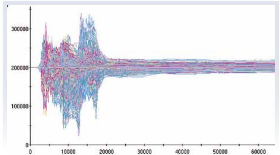
Figure: After approximately 20,000 15-minute training data records (208 days), the regression coefficients and therefore the model also are stable for the future.
