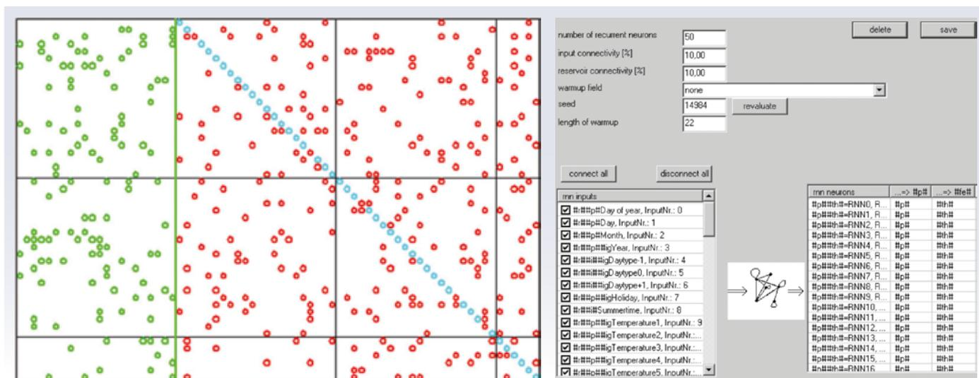
Figure: This adjacency matrix generates 50 new RNN inputs (blue) based on 27 model inputs (green).
